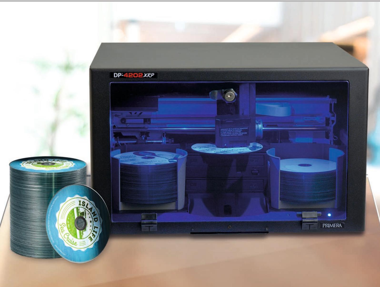
**DP-4202 XRP** automates the process of burning and printing quantities of recordable CDs, DVDs and Blu-ray Discs. Using built-in robotics, discs are transported one at a time into either single or dual optical drives. After data is burned, the discs are transported to a high-speed, high-resolution full-colour disc printer.
